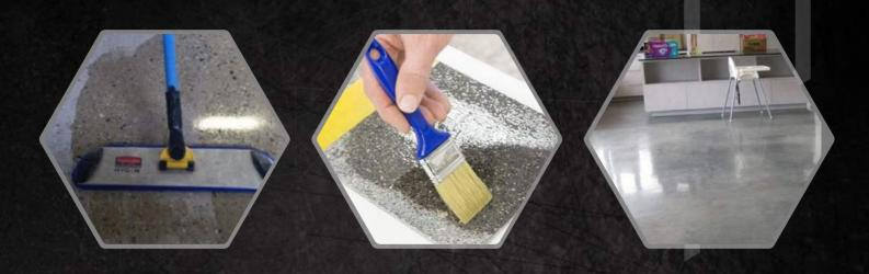
Applying the **FLOORSIL PRO** should be done by rubbing or painting with a roller. Two layer are necessary. After application the first layer, the coating remains rough, with the second layer coating is smoothed out. The consumption of the product at the first application is  $50-150 \text{ g} / \text{m}^2$  and  $20-50 \text{ g} / \text{m}^2$  at the other.
